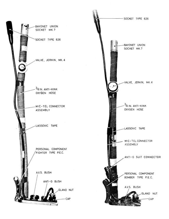
Fig. 1. Pressure jerkin hose assembly Mk. 2 Fig. 2. Pressure jerkin hose assembly Mk. 3
