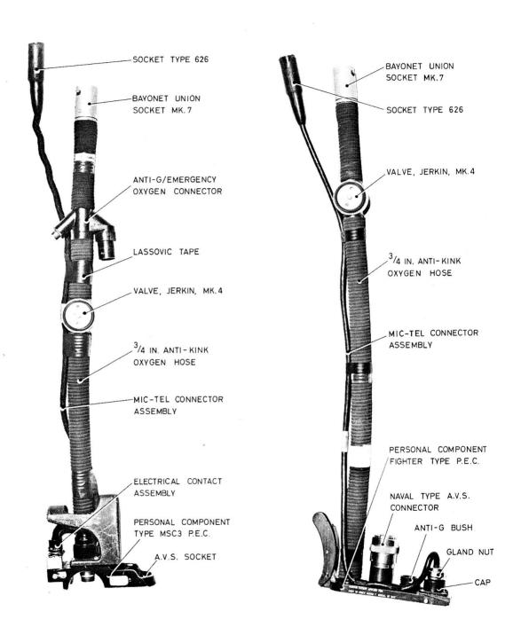
Fig. 3. Pressure jerkin hose assembly Mk. 4 Fig. 4. Pressure jerkin hose assembly Mk. 5
